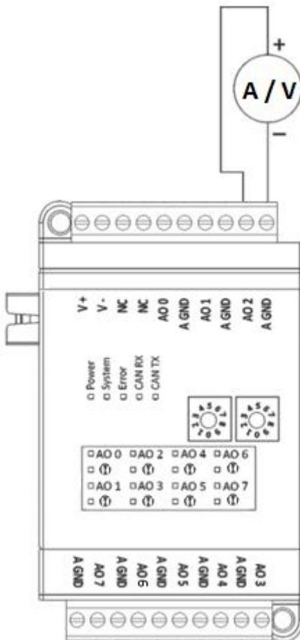
**Figure 21 Analog Output Expansion Module Connection Diagram**
