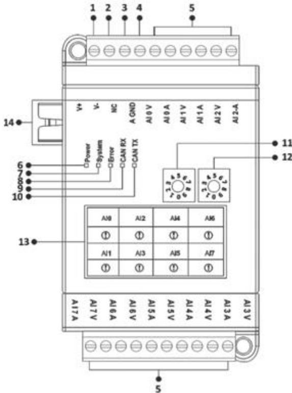
Figure 16 GD2 Board Type Connector and Physical Interfaces
