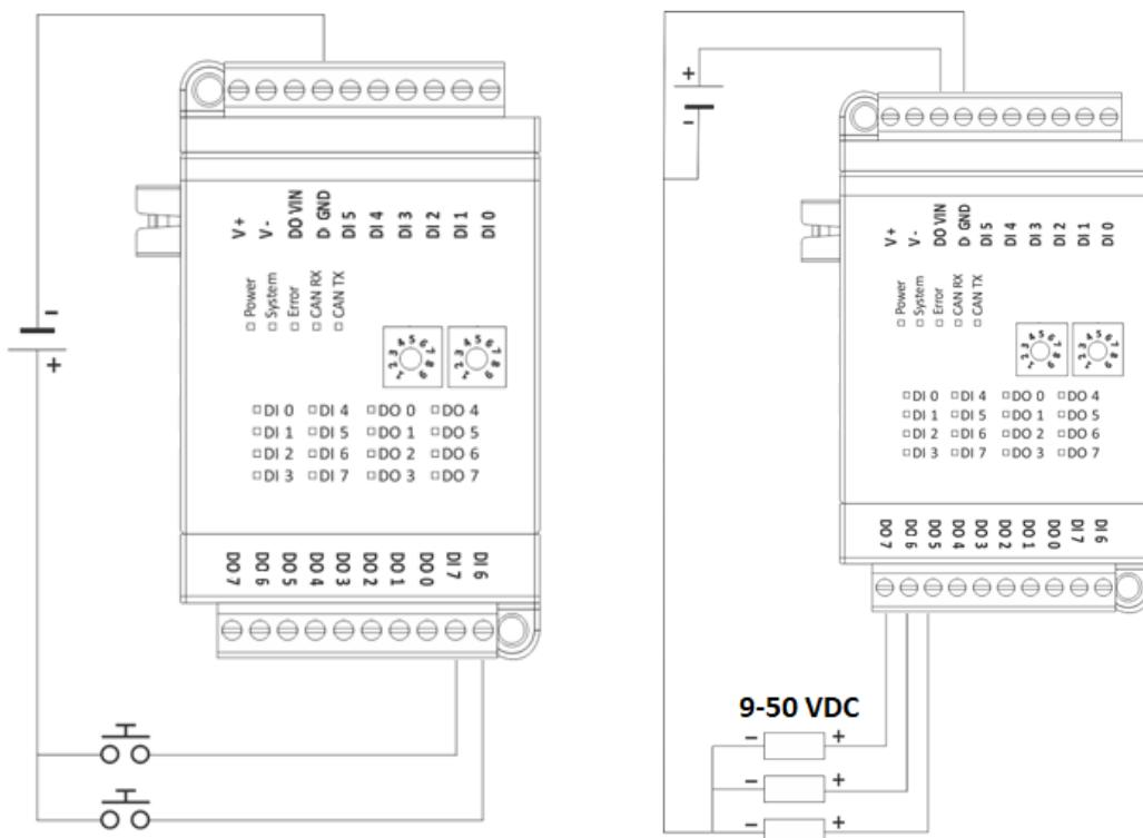
Figure 12 Digital Input Output Expansion Module Connection Diagram
