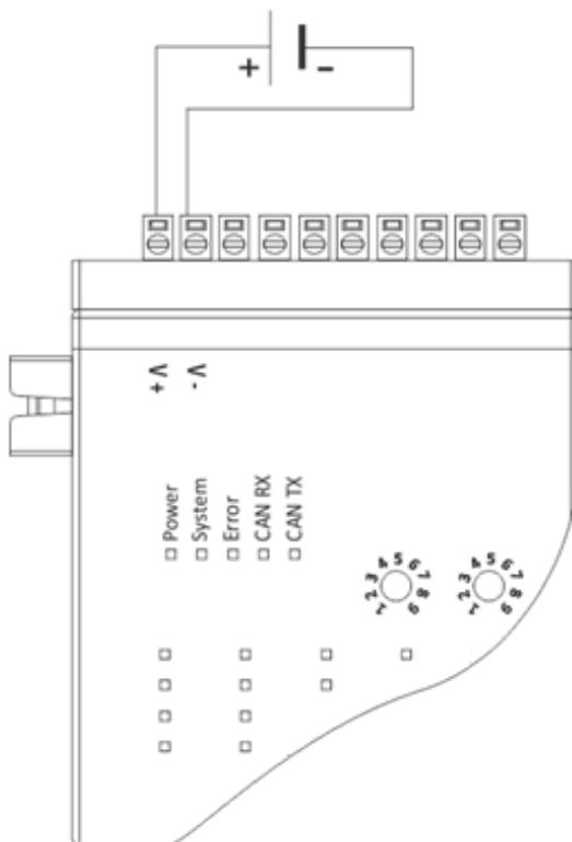
Figure 14 Relay Expansion Module Power Connection Diagram
