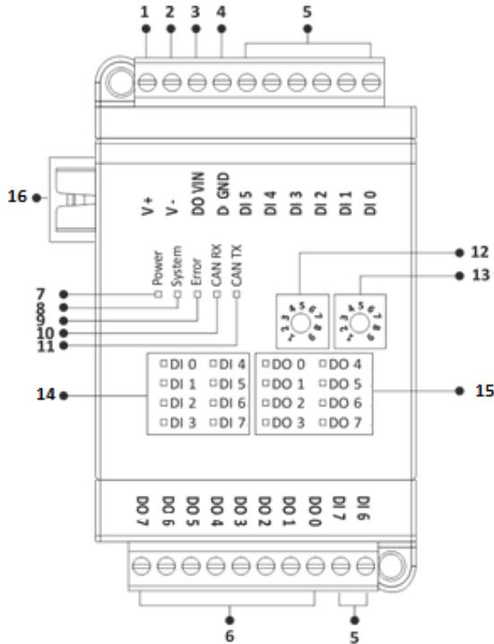
Figure 10 GD8 Board Type Connector and Physical Interfaces
