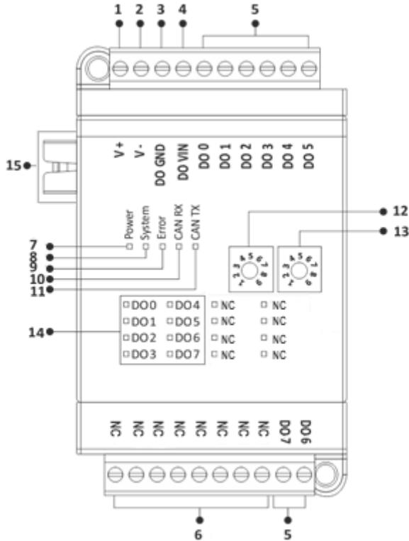
Figure 6 GD7 Board Type Connector and Physical Interfaces
