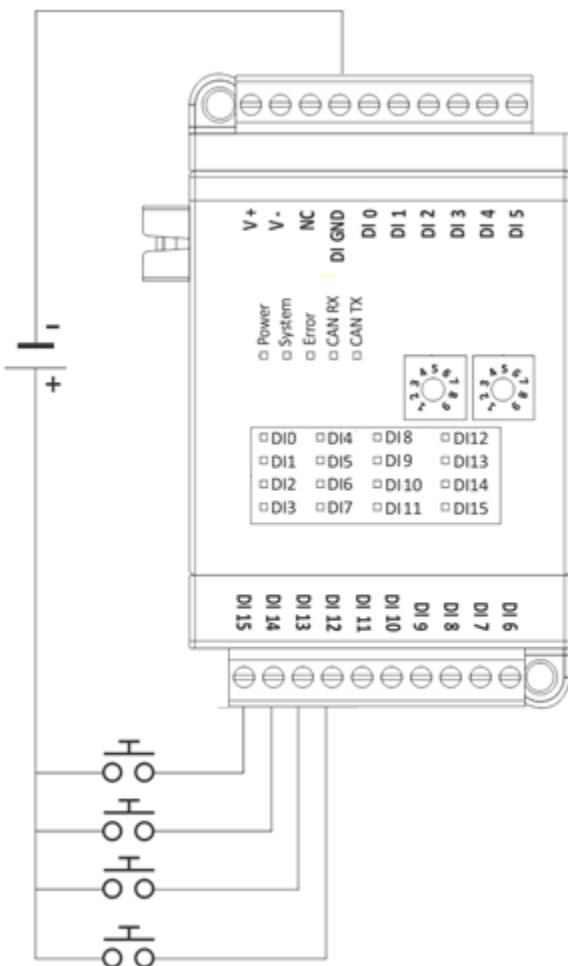
Figure 5 Digital Input Expansion Module Connection Diagram
