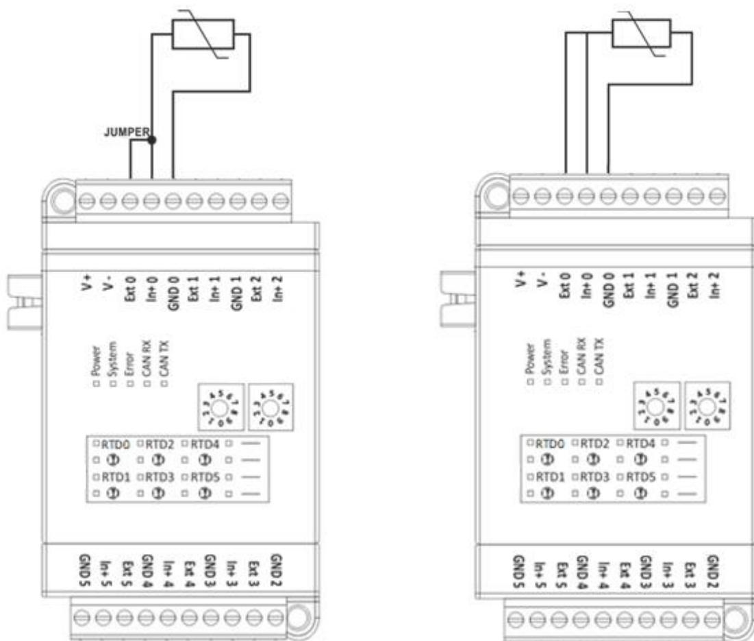
Figure 27 RTD Input Expansion Module Connection Diagram
