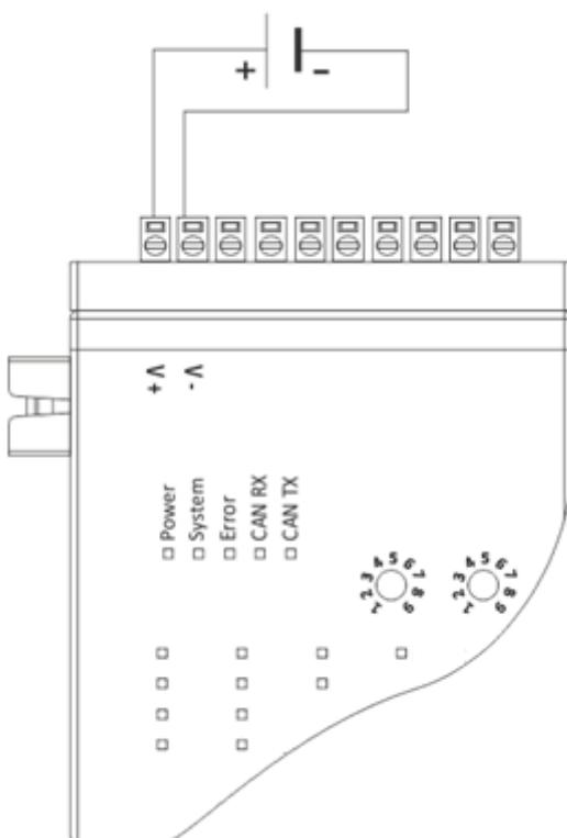
**Figure 8 Digital Output Expansion Module Power Connection Diagram**
