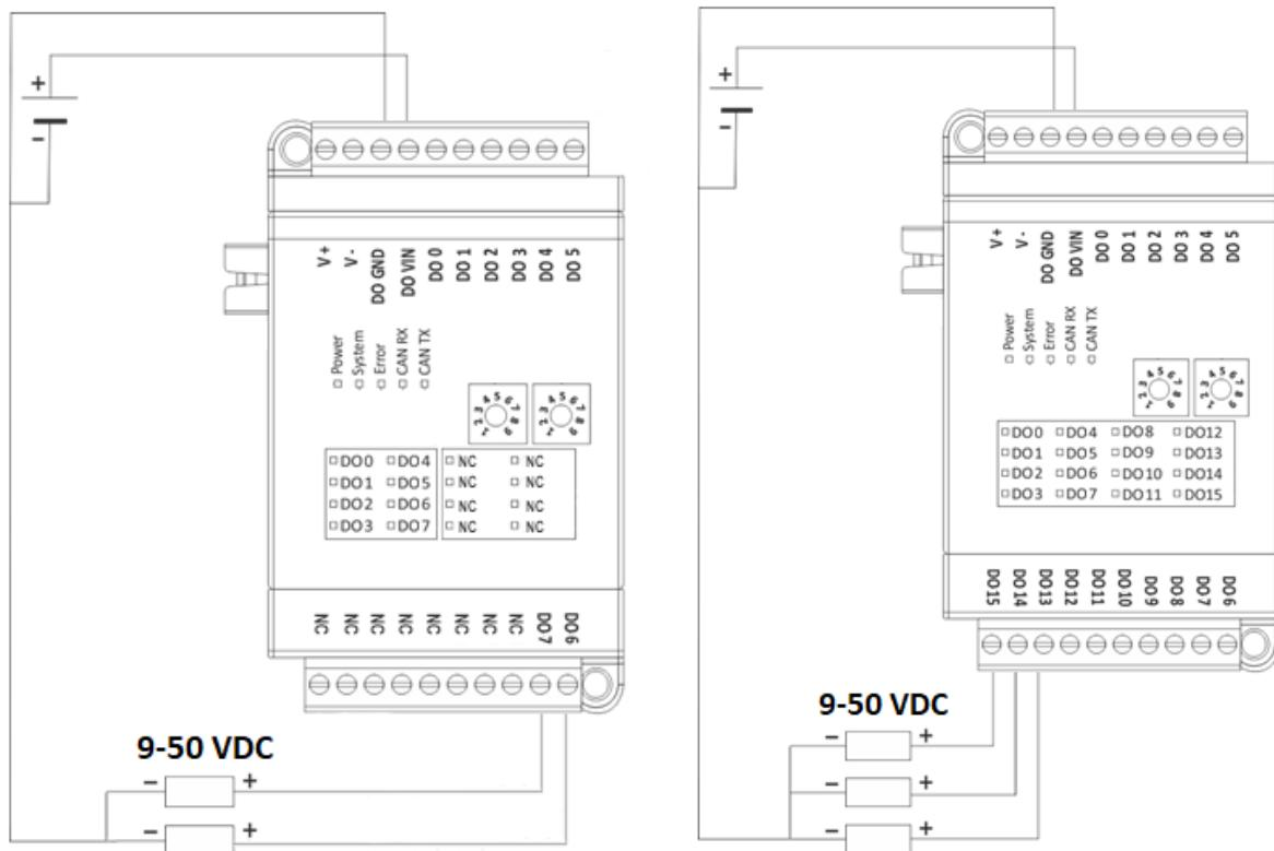
Figure 9 Digital Output Expansion Module Connection Diagram
