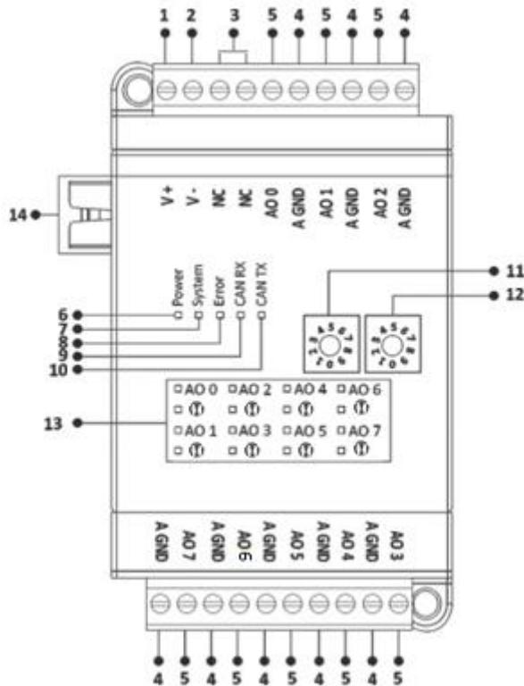
Figure 19 GD3 Board Type Connector and Physical Interfaces
