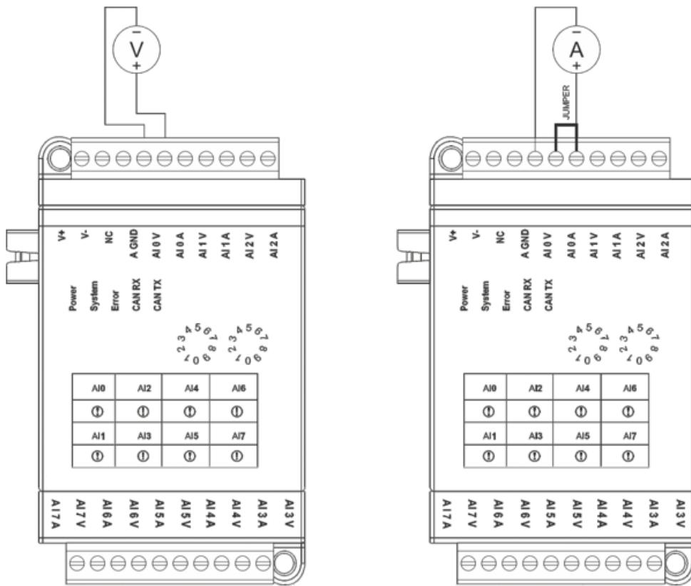
Figure 18 Analog Input Expansion Module Connection Diagram
