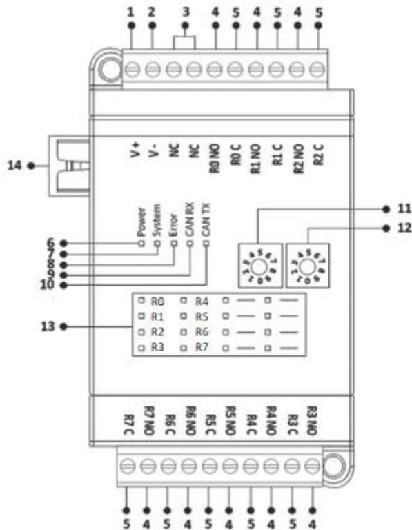
Figure 13 GD5 Board Type Connector and Physical Interfaces
