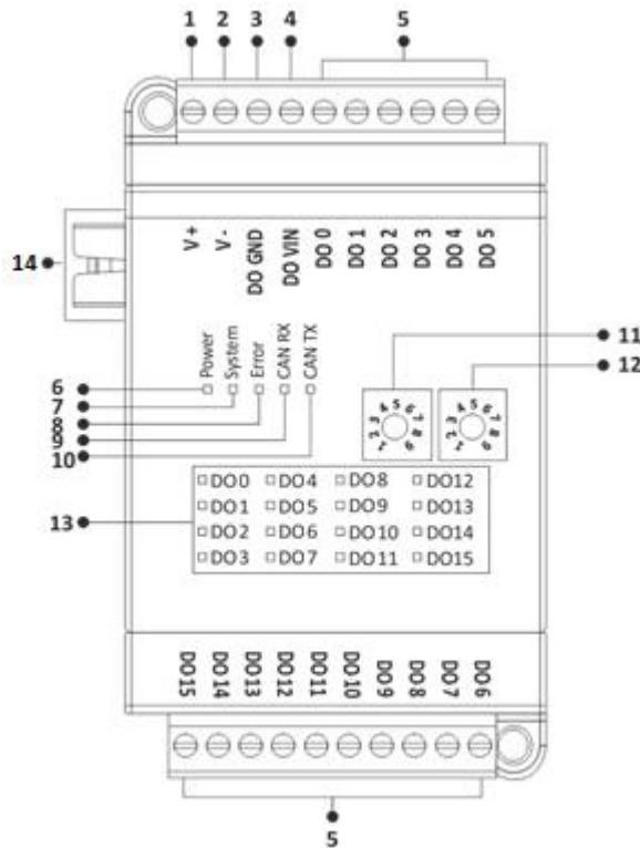
**Figure 7 GD1 Board Type Connector and Physical Interfaces**
