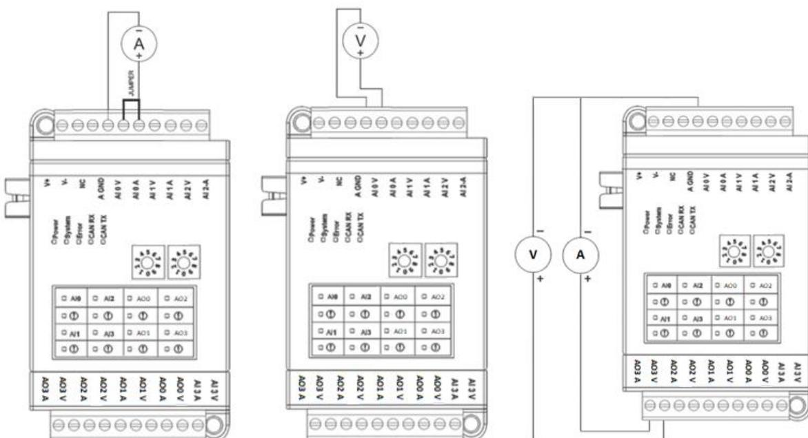
Figure 24 Analog Input Output Expansion Module Connection Diagram
