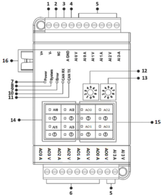
Figure 22 GD9 Board Type Connector and Physical Interfaces
