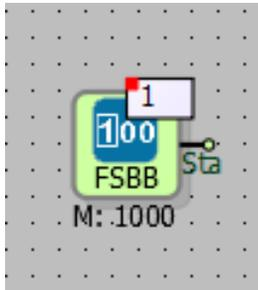
When PLC is started, the block gives logic(1) to block output.
