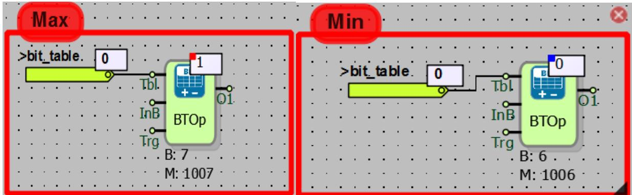
When the table has bit value 1, the maximum value is 1 and when the table has bit value 0, the minimum value is written as 0 in the block outputs.
